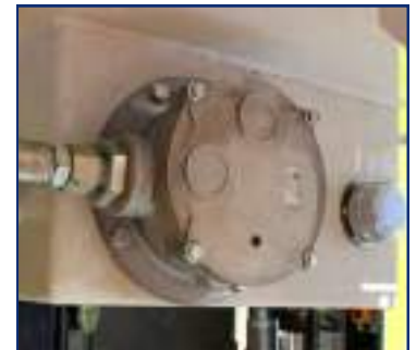
Hydraulic oil filter and oil tank breather located on top of the hydraulic oil tank
