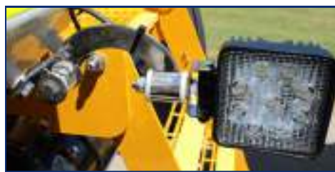
Left hand lower work light in the stationary vehicle position
