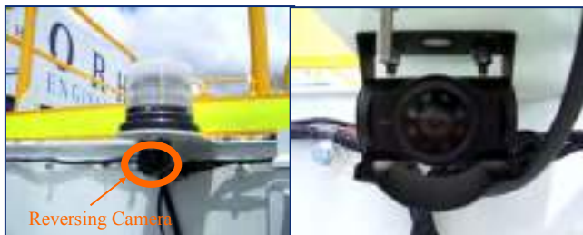
Reversing Camera Located at the top rear of the module below the amber strobe warning light /beacon
