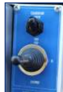
Water Cannon control panel located at the right hand side of the vehicle cabin center console.
