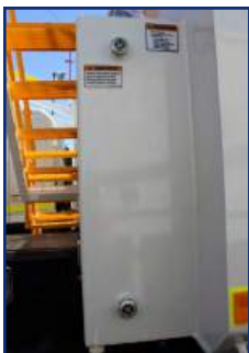
Hydraulic oil tank located at the front left hand corner of the module
