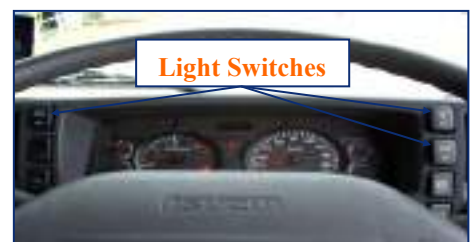
Work / inspection light switches located to the left and right of the instrument cluster
