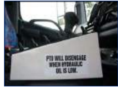
The PTO will disengage if the hydraulic oil level is low
