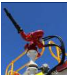
Water Cannon Located at the top rear of the water cart module.
