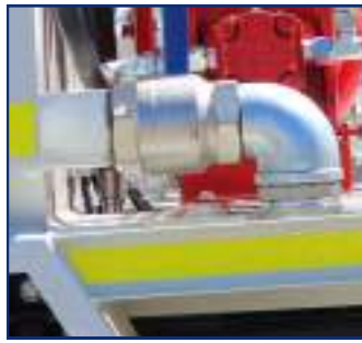
Left hand rear fill/drain point
