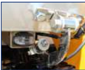
Right hand lower work light in the travelling/storage position
