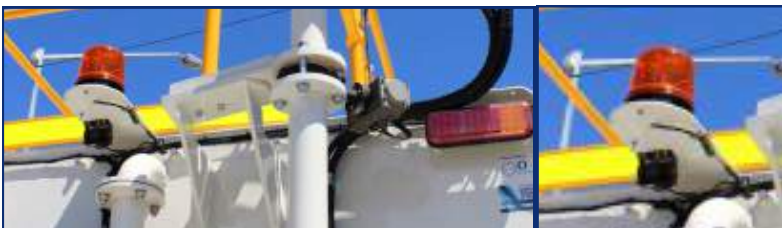
Amber strobe warning light/beacon fitted to the top rear of the module
