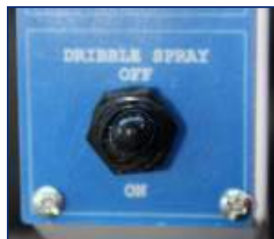
Dribble Bar switch is located along the right hand side of the vehicle cabin center console
