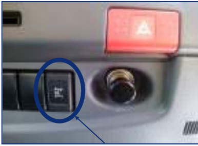
Water system PTO switch located to the left of the hazard lights switch
