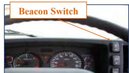
Beacon switch located to the right of the vehicle cabin instrument cluster
