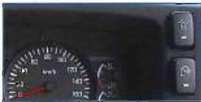
Work / inspection light switches located to the right of the instrument cluster. Top switch operates the beacon light, lower switch operates the work lights.
