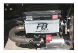
• Battery isolation switch on Compressor.
