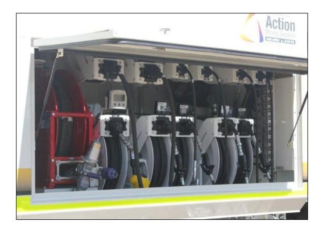
Uncoil the hose reel to desired length. It can be locked by means of the latch mechanism which is a clicking noise heard after each half resolution of the drum. By gently pulling the hose until the clicking noise has stopped, the latch is released and the hose is automatically recoiled.
