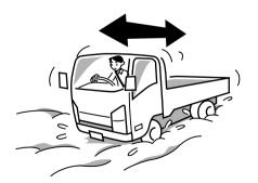
Pressing the accelerator pedal will dig the vehicle deeper into the mud and make it harder to extricate.
