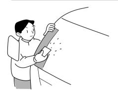
To maintain an adequate field of view, use a plastic scraper to remove snow and frost from the glass surfaces. By using a plastic scraper, you can remove the snow and frost without scratching the glass. At this time, check whether the wiper blades are frozen onto the glass.
