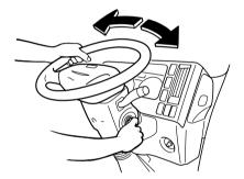
LOCK : In this position, the key can be inserted or removed.
