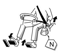
Depress the clutch pedal fully, and after waiting for a short time, press the PTO switch.
