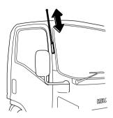
Pull the antenna out to its full length when using it.
