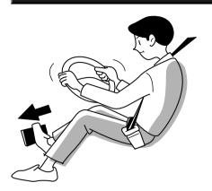
As the brake booster will no longer operate, brake effectiveness will be reduced. If the engine cannot be started, promptly have the vehicle inspected and repaired by the nearest Isuzu Dealer.
