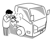
If you try to force the key into the door, you could bend it. And if you try to pull the door open with undue force, the rubber seal around the door could come unstuck or become damaged. Use warm water to melt the ice, then quickly wipe it away and open the door.
