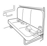
The tools are stored under the rear seat. To take out the tools, remove the seat cushion by pulling up the front.
