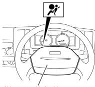
Airbag assembly for driver seat
