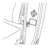
The ID plate at the lower part of the lefthand door striker indicates the chassis number together with other information such as the vehicle model code.
