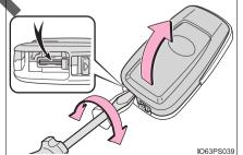
3 Remove the depleted battery.
